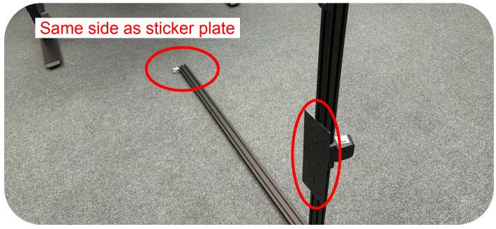
Attach sticker plate to 890mm bar using (4x) M3x6mm Button Head Bolts. Ensure the sticker is mounted right-side-up.
