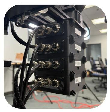
Connect the M12-RJ45 Ethernet cables to the controller boxes and Ethernet Switch. Connect the RJ45 Male to Male Cable into the Ethernet Switch.
