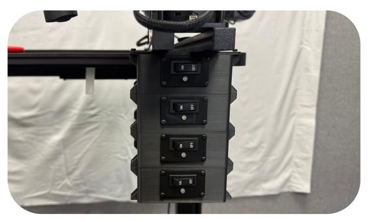
Assemble the cable management basket. Mount the cable management basket on the right side or underside of the table.
