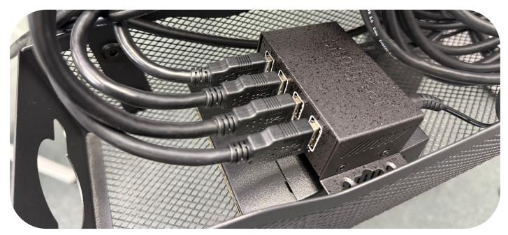
Mount touchscreen with (4x) M4x6mm Button Head Bolts. Plug the Mini-HDMI to HDMI cable into the touchscreen. Plug the USB-C Male to Male cable into the touchscreen.
