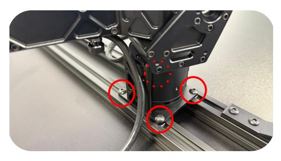
Bolt the leaders to the ends of the 1000mm bars using (8x) M5x10mm Button Head Bolts.
