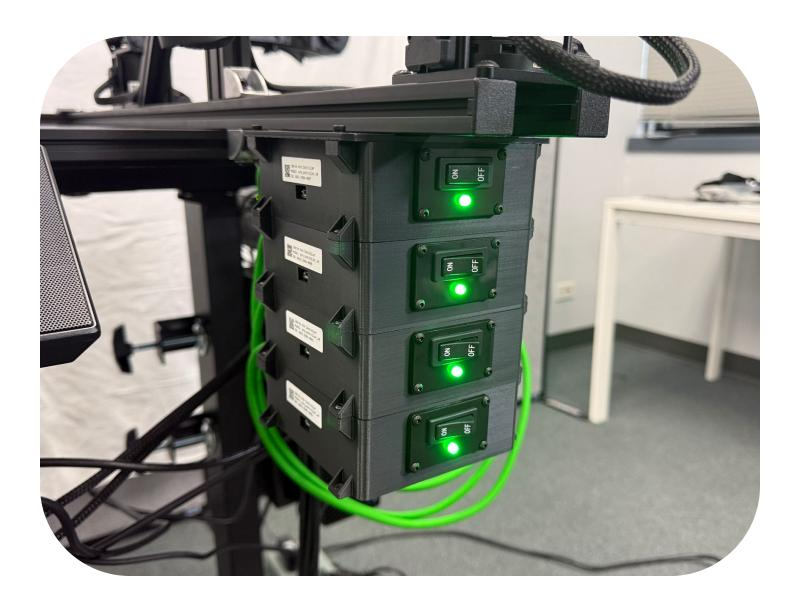
Tie up and manage any loose cables using the zip ties, 2020 cable clips, and 2040 cable clips. Ensure the arm camera cables have enough slack for full range of motion before securing the zip ties.
