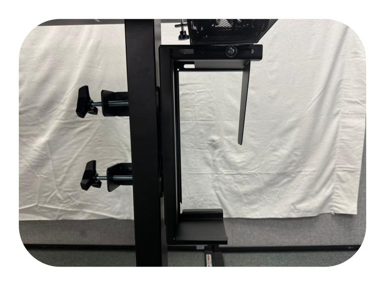
Mount the CPU in the table leg mount. Plug the CPU power cable into the CPU and power strip.
