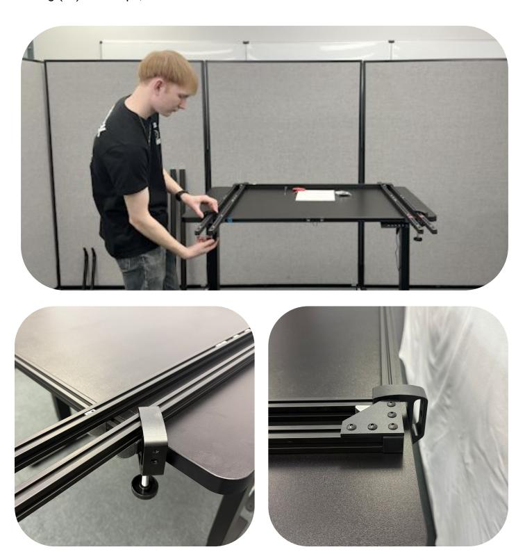
Bolt the worms-eye camera bracket to the front bar using (4x) M5x8mm Button Head Bolts. Install the lower camera in the bracket using (2x) M3x8mm Socket Head Bolts. Ensure the camera port is accessible when mounting the camera.
