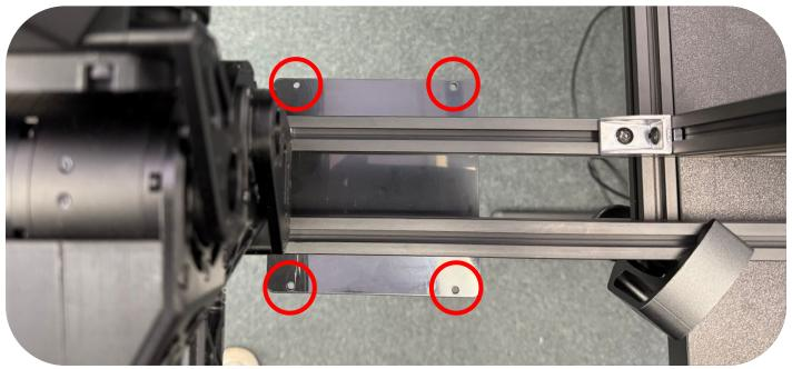
Bolt the controller tower to the lid using the (4x) M3x6mm Socket Head Bolts from step 16.
