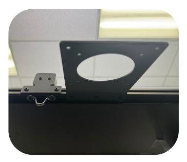
Bolt the birds-eye camera bracket to 890mm using (4x) M5x8mm Button Head Bolts. Mind orientation of camera bracket. (See Bottom Left)
