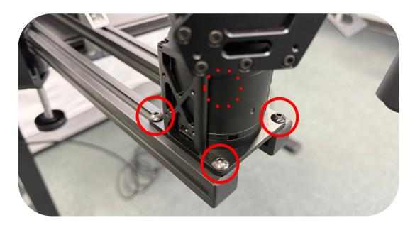
Remove the lid from the controller tower by removing the (4x) M3x6mm Socket Head Bolts. Set bolts aside to use later.
