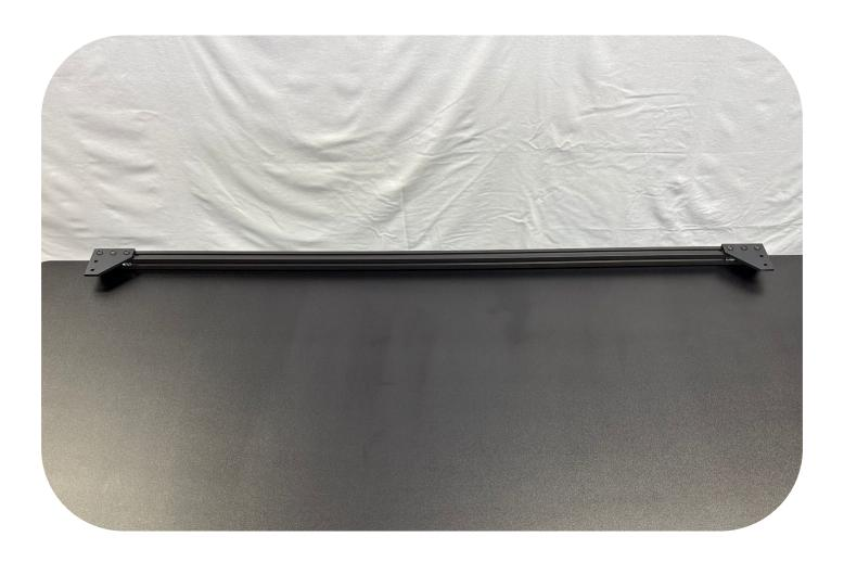
Layout the 2020-1000mm Inner Bars. Bolt the L2 + R2 bars to the rear 2020-990mm bar using (2x) M5x10mm Button Head Bolts.
