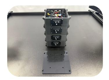
Bolt the lid under the right Leader Arm using (4x) M5x8mm Button Head Bolts. Mind the orientation of the lid when bolting it to the frame. (See Bottom Picture)
