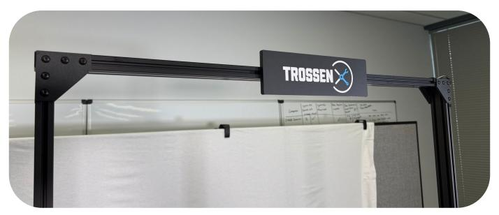
Assemble the 305mm 45 degree bars to the Upright using (4x) M5x10mm Button Head Bolts. Ensure the camera overhangs on the same side as the 305mm bars (See Red Arrow).
