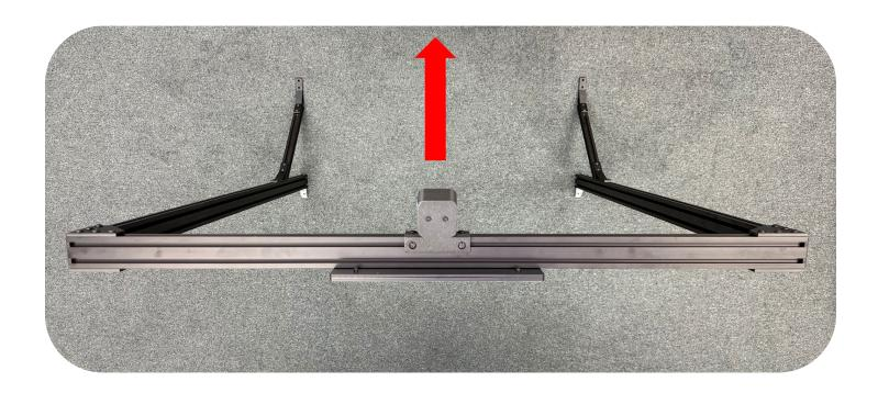
Mount the Upright to the frame using (4x) M5x12mm Button Head Bolts and (2x) M5x10mm Button Head Bolts.
