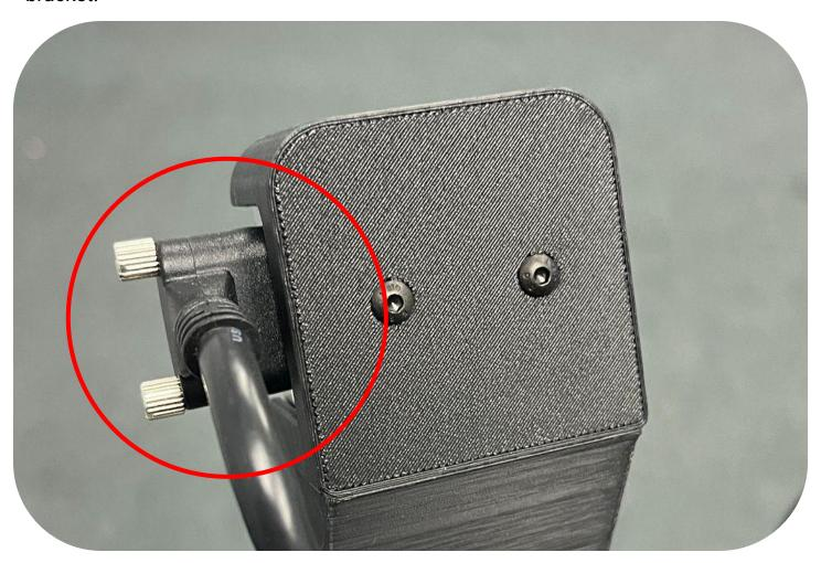
Mount the REAR WIDOWX UPRIGHT to the PODIUM and lock it into your desired height by twisting the handle clockwise.
