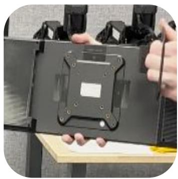
Using an M3 Driver, mount the TOUCH SCREEN MOUNT to the REAR WIDOWX UPRIGHT using (3x) M5x8b bolts.
