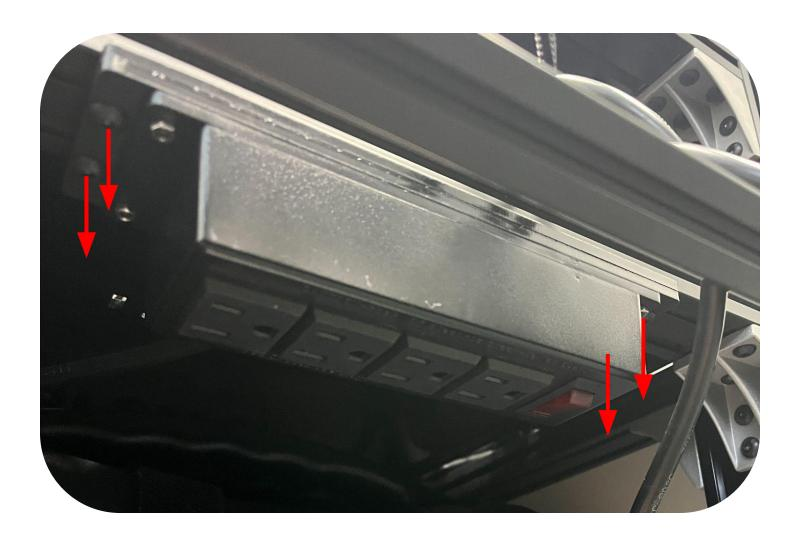
Prepare the VELCRO to insert the POWER STATION, putting the front and back velcro together into a V-shape using both ends like in the photo.
