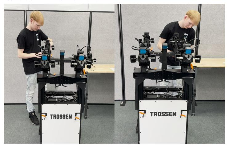
Add the CAMERA CABLE to the PODIUM CAMERA and **hand-tighten** the cable to the camera to lock it into place.
