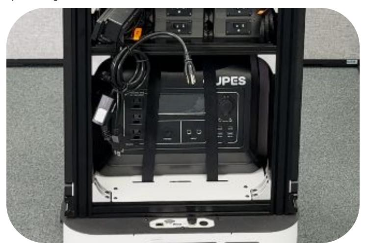
Mount the POWER STRIP under the ELECTRONIC PLATE reusing the (4x) M5x14b bolts from STEP 6.
