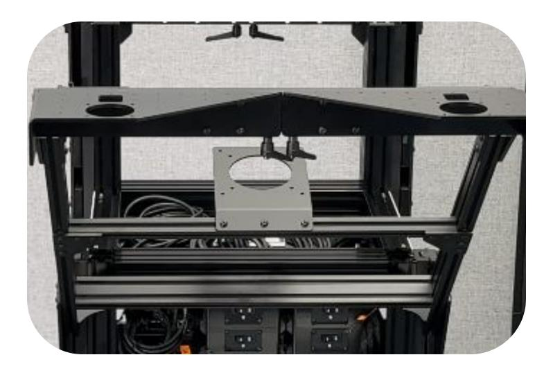
Using an M2.5 Driver, mount the TOUCH SCREEN to the TOUCH SCREEN MOUNT using (4x) M4x6b bolts.
