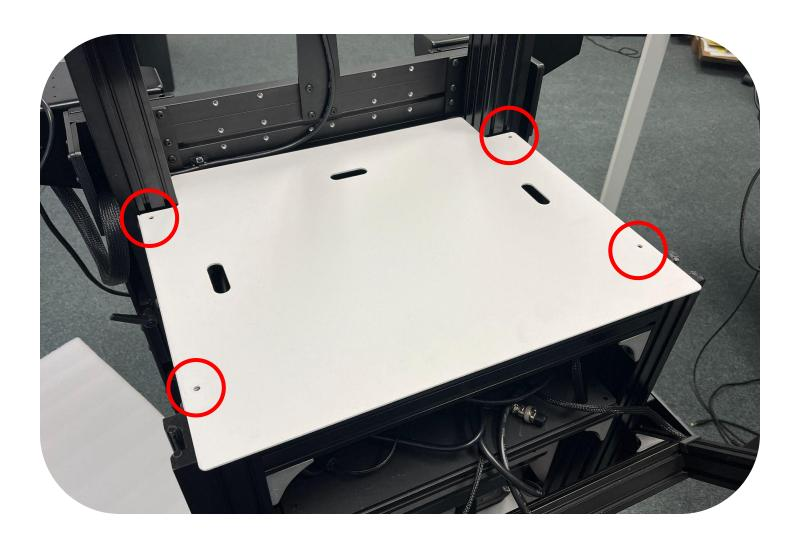
Remove the POWER STRIP using an M3 Driver and save the (4x) M5x14b bolts to reuse later.
