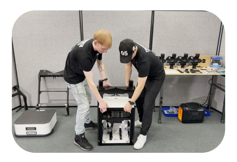
Carefully place the PODIUM on the SLATE. Mount the PODIUM to the SLATE using (12) M5x12b bolts found in the accessory bag.
