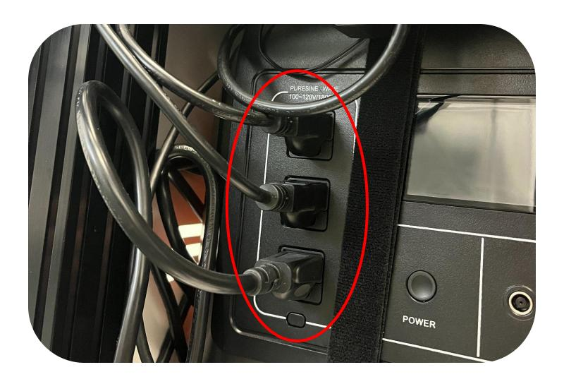
Plug in POWER SUPPLIES for both the USB HUB and the 5-PORT ETH SWITCH into the 4-PORT POWER STRIP.
