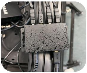
Plug in one end of the RJ45 MALE TO MALE CABLE into the 5-PORT ETHERNET SWITCH and leave the other end unplugged.
