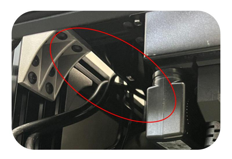
Plug in the POWER SUPPLIES for the ARMS into the POWER STATION.
