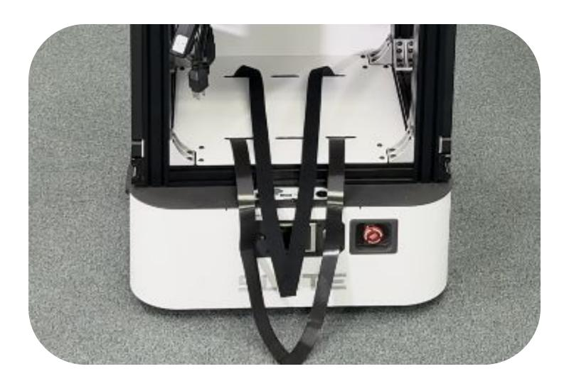
While holding on to the rear VELCRO to prevent it from getting stuck in the back, insert the POWER STATION on top of the BOTTOM PLATE.
