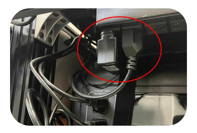
Plug in the USB-A MALE TO MALE CABLE into the SLATE and into the USB HUB.
