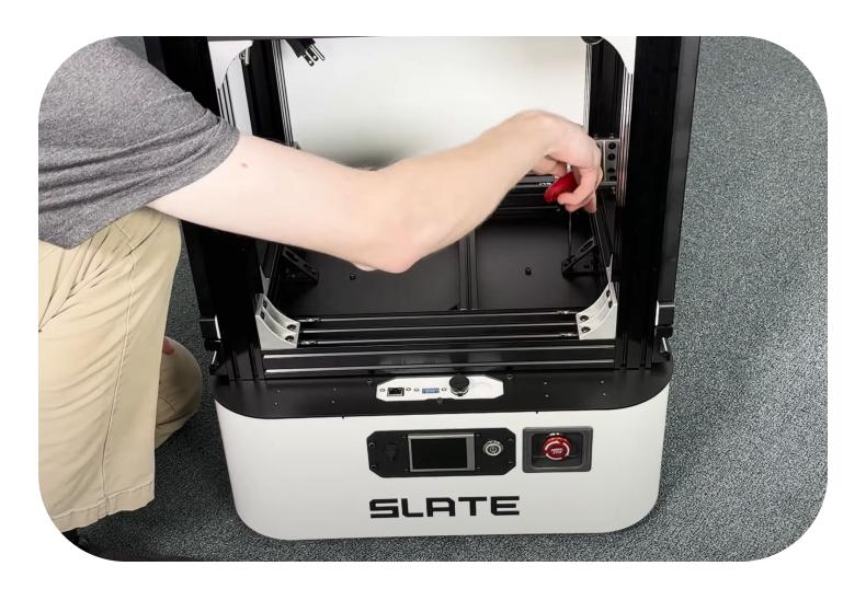
Mount the POWER SUPPLY PLATE to the bottom layer of the PODIUM using an M3 Driver for the (12x) M5x8b bolts.
