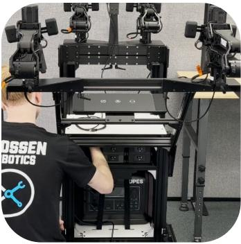
Pull the USB-A MALE CONNECTOR from the USB HUB, and the RJ45 MALE CONNECTOR from the ETH SWITCH, through the LAPTOP PLATE slots for access to the Laptop on top of the PODIUM.
